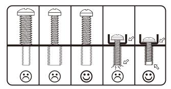
The back of your TV has 4 screw holes in a square or rectangular pattern. This is where the mount will attach to your TV. Kanto provides several sizes and lengths of screws. This guide will help you select the right screws for your TV. You will only use 4 of the provided screws to attach your TV – the rest are not needed.
