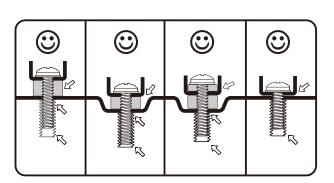
Plastic spacers are also provided in 2 thicknesses to allow the mount to work with curved TVs, and TVs that have recessed mount holes, protrusions, or inputs in the way. They can also be used to prevent the TV screws from going too deep and damaging your TV. You may not need spacers for your TV.
