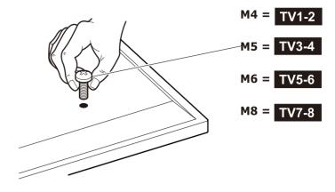
You are provided with 4 diameters of TV fixing screws, **M4**, **M5**, **M6** and **M8**. Determine the screw diameter that fits.
