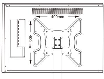
VESA large than 200x200 and small than 400x400, it should be install the extensions.
